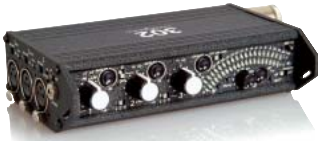
The Sound Devices 302 mixer packs a lot of features and great audio performance into a 1.8-pound (with batteries) package.
