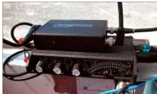
The 302 works great in an audio bag, but is so small that you can use it in many ways. The compact size came in handy when I had to rig the mixer to fit in a small research aircraft.
