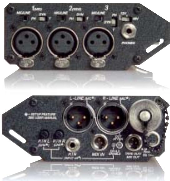
Each of the 302's three transformer-balanced XLR inputs (top) accepts either mic- or line-level signals and has its own peak limiter. The two line/tape/mic-level XLR outputs (bottom) are active balanced.
